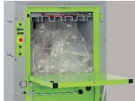
Compaction of plastic material (foil)
