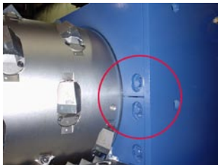
Replaceable wear plate inside chamber
