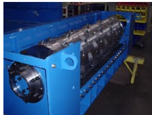
Modular rotor design allows for offline maintenance in applications where downtime is critical
