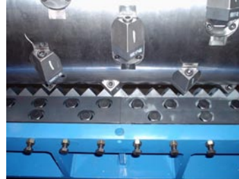
Anvil tolerance adjustments are easily accessed and simple to perform. Anvil-to-cutter tolerance is a critical factor in the success or failure of many applications
