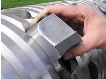
Removable cutter holders allow flexibility in cutter placement (versatility in application changes) as well as easy replacement in the event of failure (no welding)
