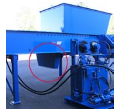
Drop out zone behind ram for reduced maintenance
