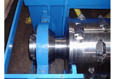
Unique outboard bearing design with dual drop-out zones and mechanical labyrinth at the rotor help keep contaminants away from the bearings, which prolongs bearing life
