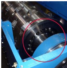
Rotor investment protected with bolt-on stub shaft on drive end
