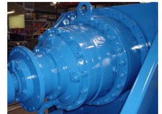
Planetary gearbox is mounted directly onto rotor. This allows larger rotor output shaft and much more gear surface area contact, which means more service factor
