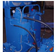
The "Max Force" HPU with a pressure compensated pump-ram force controlled by rotor current
