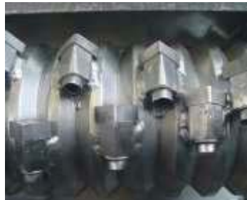
Profile rotor with welded knife carriers
