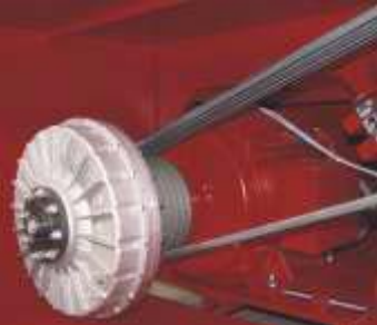
Transmission and hydro coupling
