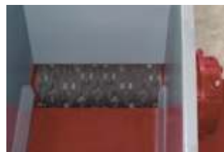
GAZ 82 S with a large rotor diameter of 368 mm. This allows for a high throughput capacity.
