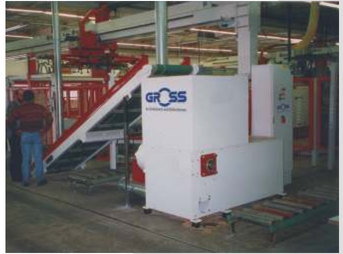
GAZ 82 with customer specific hopper (sound proofed, double skinned)
