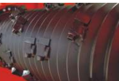
Profile rotor with a diameter of 368 mm and concave knives
