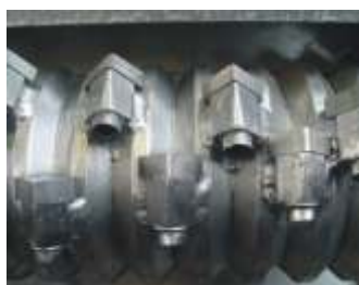
Profile rotor with a diameter of 252 mm and flat knives
