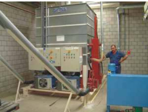
Briquette press GP 150 with two briquetting units for higher output
